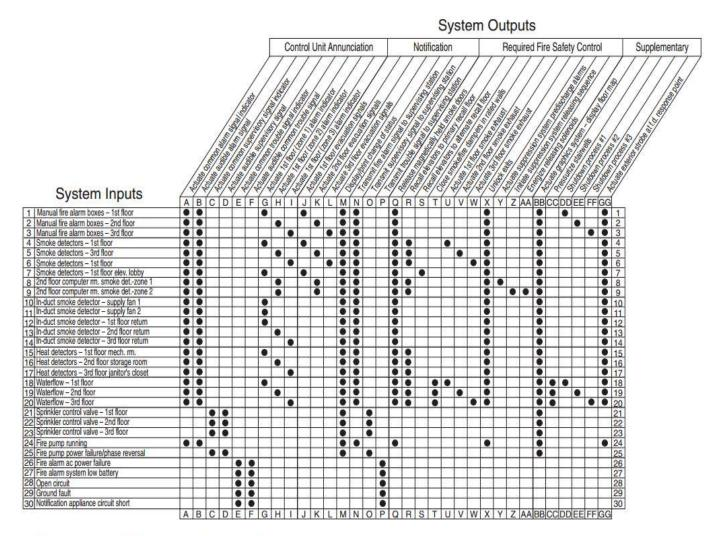
FIGURE A.14.6.2.4 Typical Input/Output Matrix.
